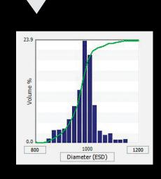
The two particles below have the same size (ESD) according to volumetric-based particle analysis techniques, like laser diffraction and light obscuration, but are clearly different. Dynamic imaging particle analysis allows you to see what's under the curve - both shape and size of your particles - providing you with microscopic particle measurements which enable you to separately count different particle types in the same sample.
